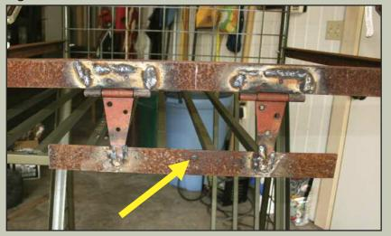
A %-inch metal drill bit was used to drill this small hole into the trigger mechanism so that it can be attached to a trip wire.
