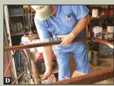
A piece of angle iron marked for cutting (A). After cutting (B and C), the iron can be heated and bent to form the desired configuration (D). The bracket is then welded. Designs may differ, depending on the door style.
