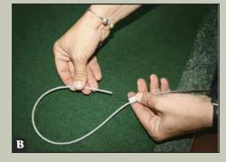
Create an adjustable end by sliding a double ferrule over the cable (A) then feeding the cable back through the double ferrule.
