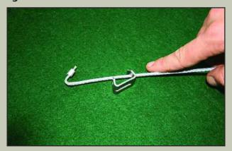
Reverse bend above single ferrule to secure the snare lock.
