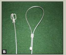
Attach a ferrule to the end of the cable (A). The snare can be designed with a swivel end (B-left) or an adjustable end (B-right).
