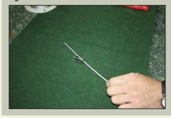
Run the cable through the snare lock.
